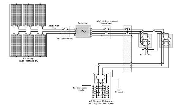
N.B this drawing is intended for illustration purposes only in the application for interconnection and does not represent a design or installation manual
